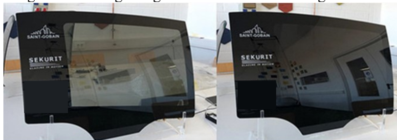
Figure 2: Visual appearance of a guest-host liquid crystal sidelite prototype in transparent and tinted state.
